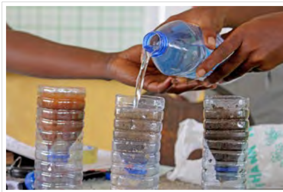
Figure 107. Testing water retention
